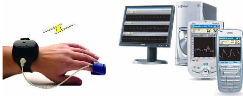
Figure 3.4 - A wireless oximeter based monitoring system
